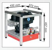
Operating pressure 630 - 720 bar Oil flow/Pressure 2 x 2.4 l/min / 180 bar 2 x 0.9 l/min / 720 bar Power unit 4-cycle gas engine 2.7 kW Power Oil tank (usable amount) 7.5 (6.5) | Width/Depth/Height 432 / 372 / 457 mm Weight approx. 33 kg Order-No. 74500
